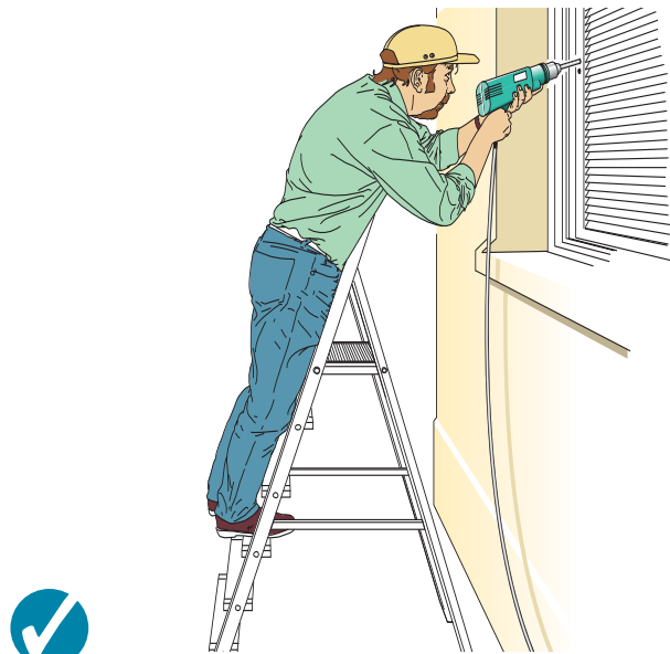
Figure 2b Correct - steps facing work activity
